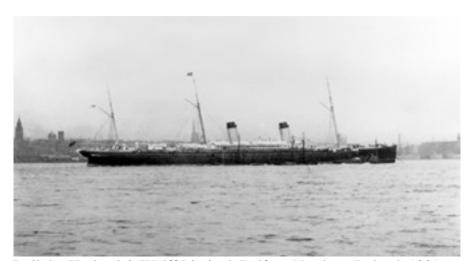
Built by Harland & Wolff Limited, Belfast, Northern Ireland, 1889. 9,686 gross tons; 582 (bp) feet long; 57 feet wide. Steam triple expansion engine, single screw. Service speed 20 knots. 1,490 passengers (300 first class, 190 second class, 1,000 third class). Two funnels, three masts.
